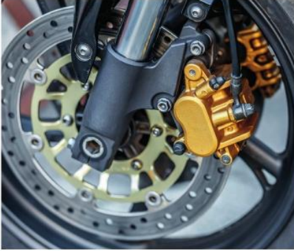
▲ Figure 3.8 Motorcycle disc brakes work using friction. Friction is necessary if we want things to stop.
