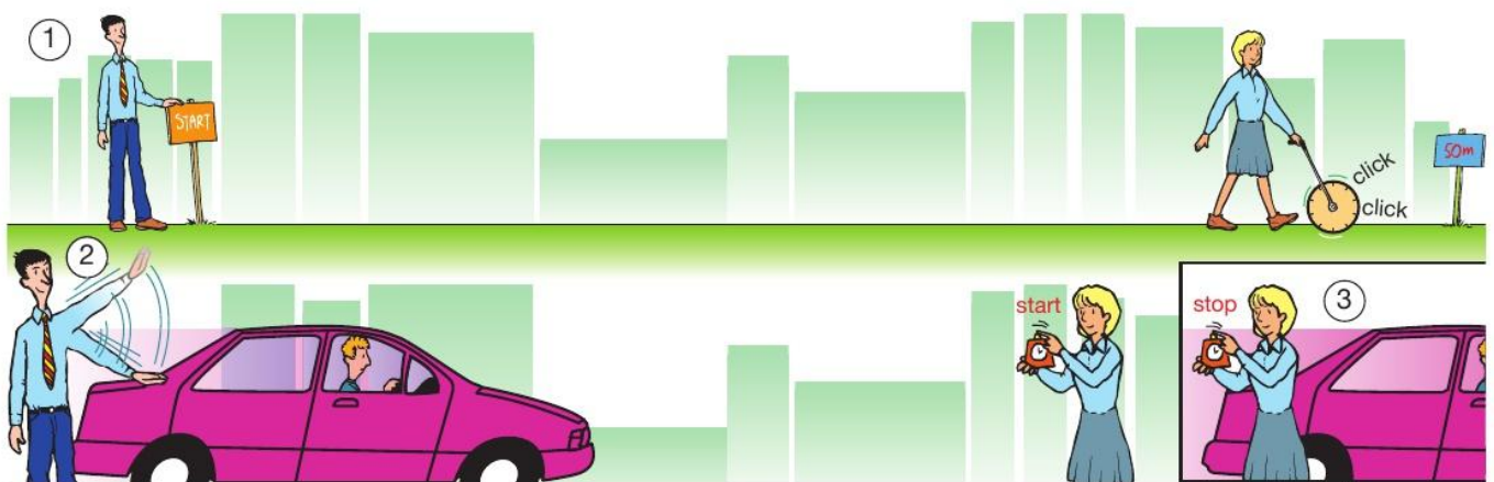
▲ Figure 1.4 How to measure the speed of cars driving on the road
