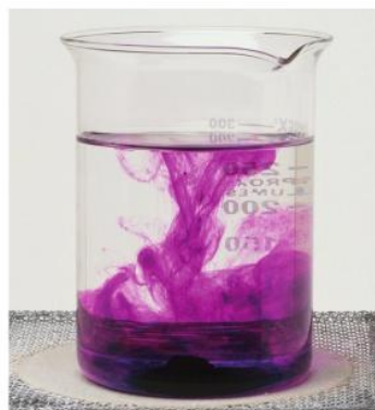
▲ Figure 15.4 Demonstration of convection currents, using a potassium manganate (VII) crystal in water
