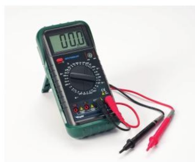
▲ Figure 7.3 An ammeter is used to measure current in a circuit. It has a very low resistance and so has almost no effect on the current.
