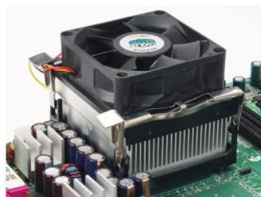
▲ Figure 15.13 a A shiny kettle stays warmer longer. b The heat sink needs to be matt black to lose heat to the surroundings quickly, and so stop the transistor overheating.
