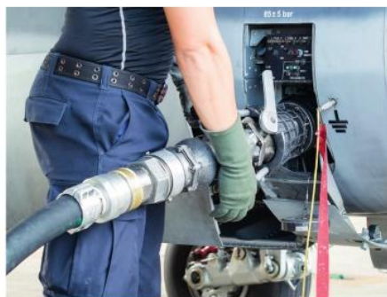
▲ Figure 9.17 Earthing during refuelling
