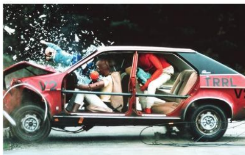
▲ Figure 4.7 Parts of cars are designed to crumple.
