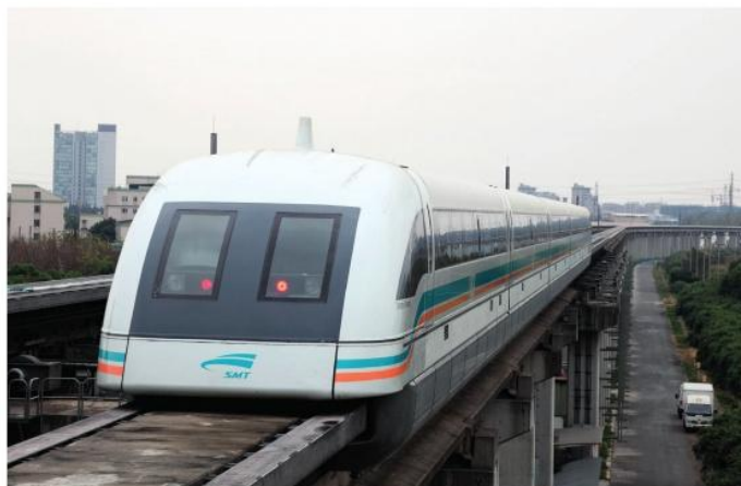
▲ Figure 8.20 Maglev trains use superconducting magnets to help them hover above the tracks.
