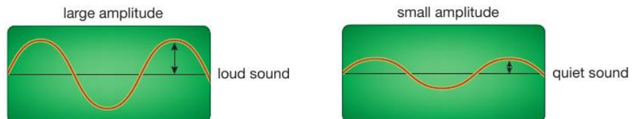
▲ Figure 13.13 Loud sounds and quiet sounds on an oscilloscope
