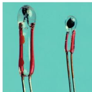
▲ Figure 8.14 Two examples of thermistors and their symbol – the resistance of a thermistor changes a lot as the temperature changes.
