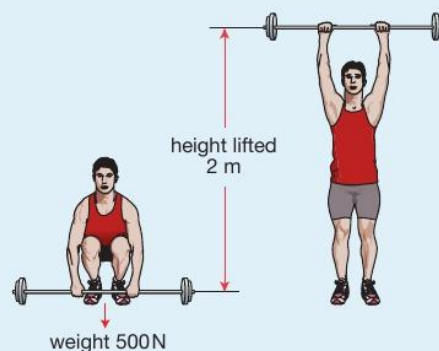
▲ Figure 16.2 Doing work by lifting a weight
